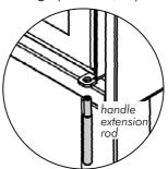
We recommend you wear the gloves provided with the heater or the handle extension rod to open the door.
