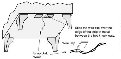
Feed the two snap disk wires into the eye of the wire clip. Then carefully remove all slack from the wire, making sure not to dislodge the snap disk. Pinch the eye of the wire clip to secure the wires.
