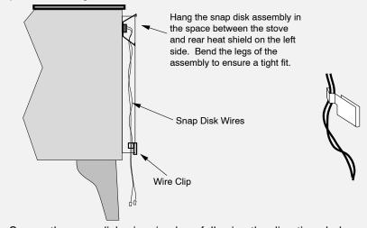
Feed the two snap disk wires into the eye of the wire clip. Then carefully remove all slack from the wire, making sure not to dislodge the snap disk. Pinch the eye of the wire clip to secure the wires.
