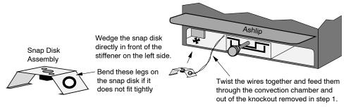
2A Secure the snap disk wires in place following the directions below. Go to step 3.
