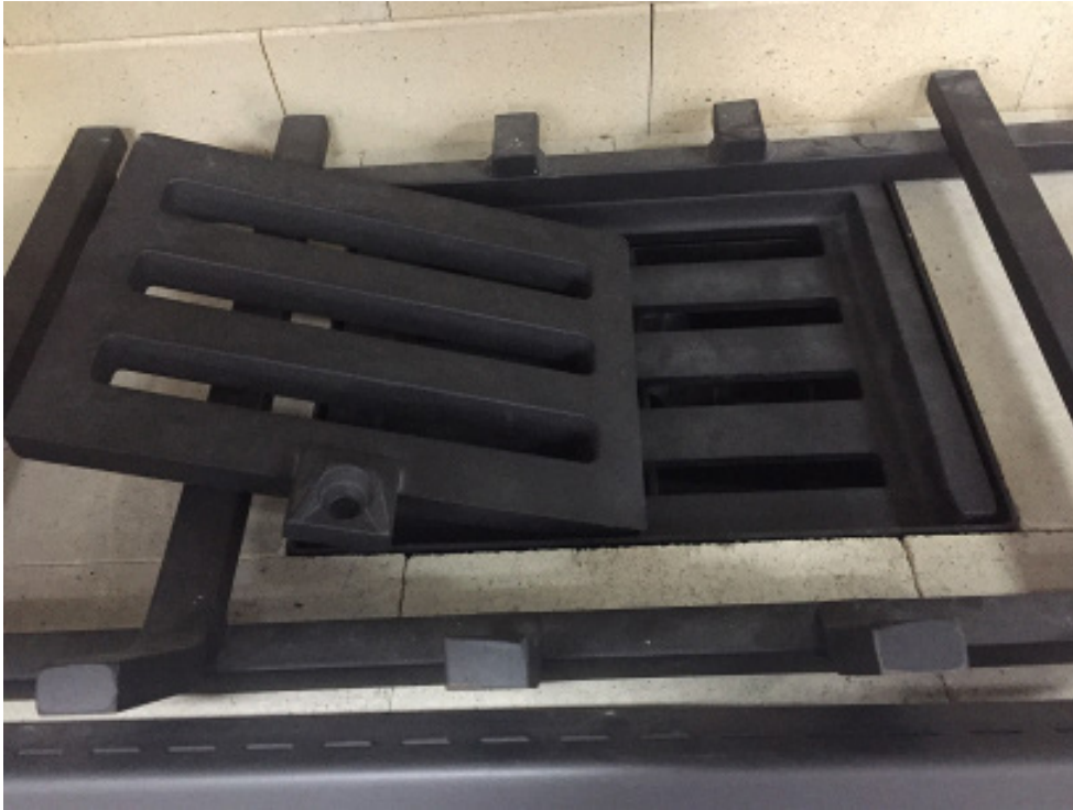
Figure 1. Larger Ash Grate pictured with smaller grate offset to larger grate
