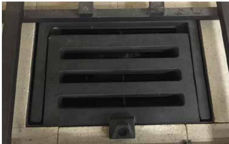
Figure 2) Smaller Ash Grate pictured inside the larger Ash Grate. Also shown in fully-open position.
